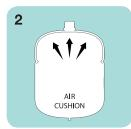
Install the expansion tank on the supply side of the water heater, on the suction side of the geating circulator.
