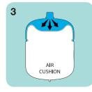
Once the expansion tank is installed, re-pressurize the system and check for leaks. Repair as necessary.
