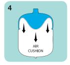
Restart the water heater system and check for relief valve discharge. If the relief valve drips, the tank may be improperly charged or undersized.
